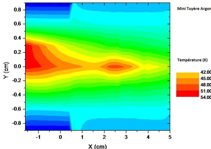
Molecular beam temperature vs position at the nozzle exit. The nozzle and X axis are the same one
