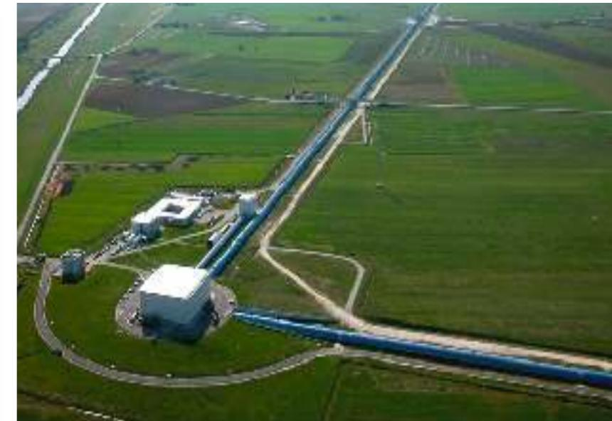
3-4 km vacuum tunnels with laser beam bouncing off of mirrors
